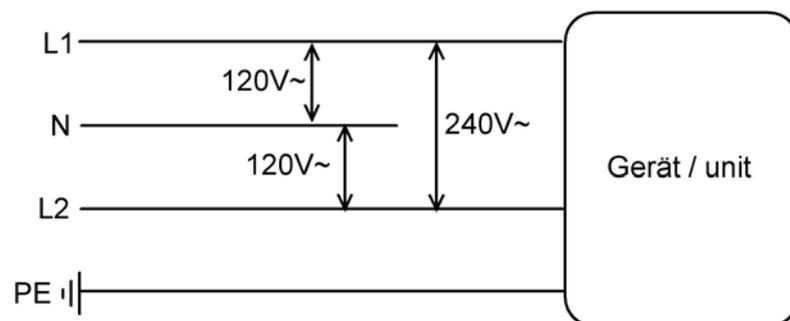
Diagram: required mains conditions for S 450 H / S 900 H in 120 V mains.
