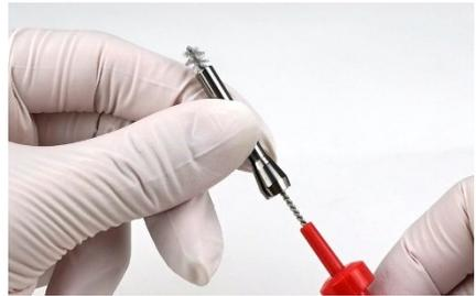
Rinse the chuck very well, and make sure you let it dry well afterwards. Cover your index finger with a very little amount (just a drop) of oil and rub in between your thumb and index finger. Dab off the oil until your fingers is only covered with a very thin film of oil. Now move the chuck in between your thumb and index finger. There should be only a very thin film of oil left on the chuck. Please act according to the saying: Less is more.
