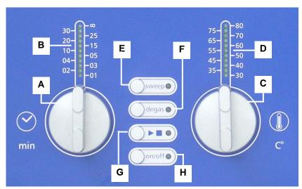
Illustration 4.7 View operating elements (unit with heating)
