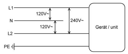
Diagram: required mains conditions for S 450 H / S 900 H in 120 V mains.
