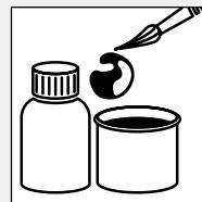
4. Varnish with hot-curing lacquer signo or air drying lacquer L, L nano or lacquer opaco
