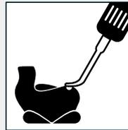
4. Level irregularities, holes or scratches with correcting wax
