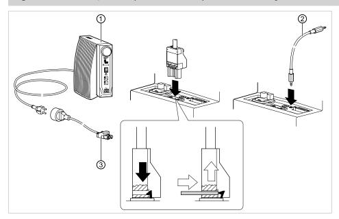
► Connect the equipment without control output ① via connection cable ③ to the SMARTair.
