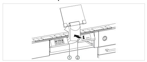
▶ When using an extraction hood ②, make sure that the intake opening ① is completely covered by the rubber lip.
