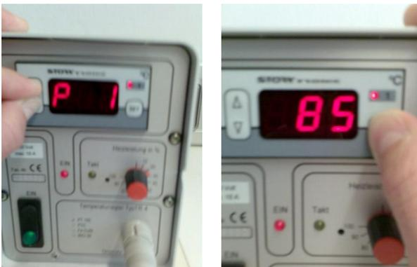
We recommend adjusting the temperature (“heating power in %”) to 25% by using the red switch!
